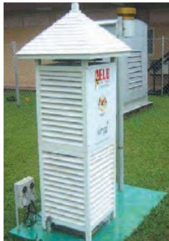
*The early warning system: Environmental Radiation Monitoring System (ERMS Detector).*
